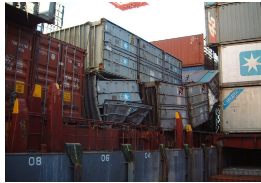
Figure 2.4: Damages on the containers. On the left, the APL China, on the right, the Dirch Maersk.
